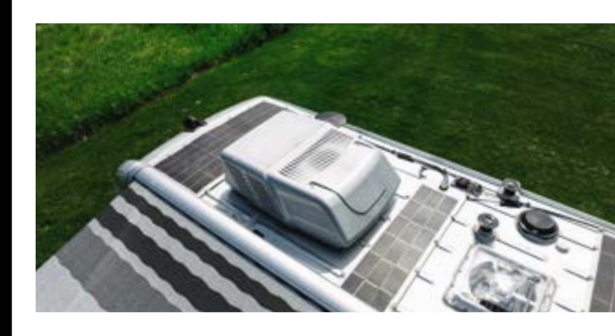
1 250 watts of solar panels on the roof harvest the free, abundant power of the sun.
