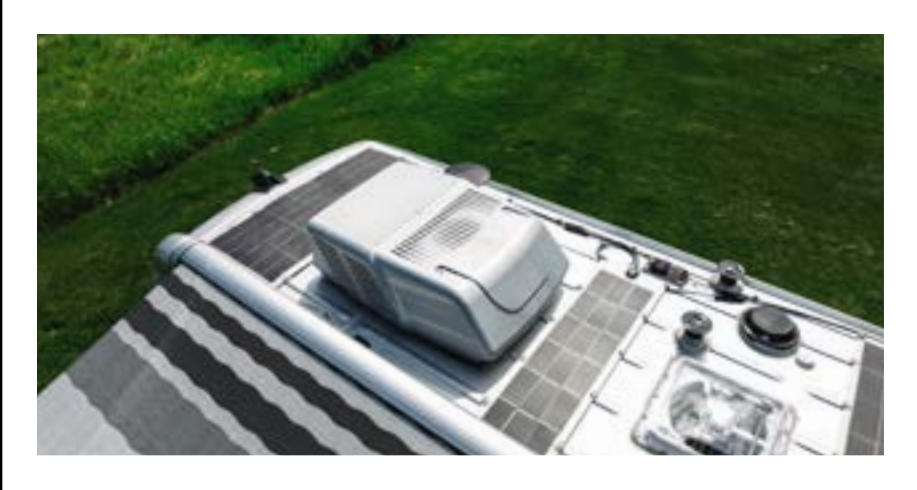
1 250 watts of solar panels on the roof harvest the free, abundant power of the sun.
